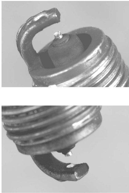
Fig. 11 Arcing pattern on platinum pin spark plug
