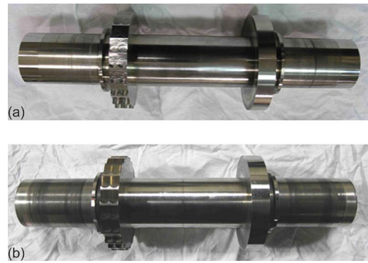
Fig. 7 Photographs of the rotor before and after misalignment tests showing edge wear in the shaft coating in photo b. (a) Rotor before misalignment tests and (b) rotor after misalignment tests.
