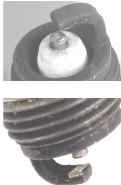
Fig. 10 Arcing pattern on heated spark plug
