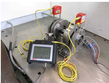
Fig. 3 Photograph of the test rig with the laser alignment system in place
